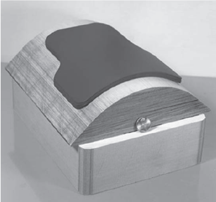
Fig. 9.45 Monolithic armor panel placed on the curved mandrel after curved layer LOM and decubing (Reprinted from Klosterman et al. 1999. With permission. Copyright Emerald.)
